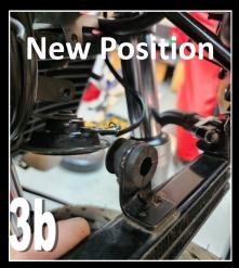
**4)** Now fit the oil cooler to the bracket using the original RC36 bolt and nut.
