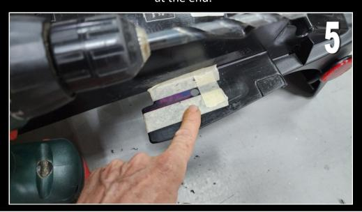
**6)** Next job is to cut up against the tape, up to the drilled hole. I used a simple 18T saw blade for this with slow careful strokes.
