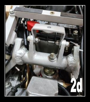
Do not fully tighten at this stage. We will need to adjust when the tank is fitted.
