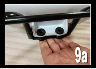
Place the tank onto the frame and rear mount and line up the holes.
