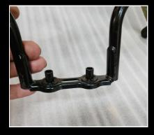
**2)** Now we need to prepare the TYBP-0009: Fitting Kit for Fuel Tank, RC36-2, RC30 Style. Fit TYLY-0347B bush to the right frame lug. This bush reduces the internal diameter suitable for an M8 bolt.
