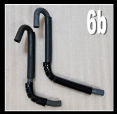
The hose can be fitted to the fuel cock after fuel tank fitting to ensure the correct routing.
