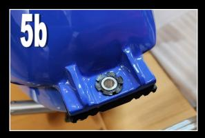
Also fit the BPSY-0345 Rubber, Tank, Side to the frame. These are held with double sided tape. Note the position relative to the weld on the frame, but I advise that you fit these first without gluing and adjust if necessary.
