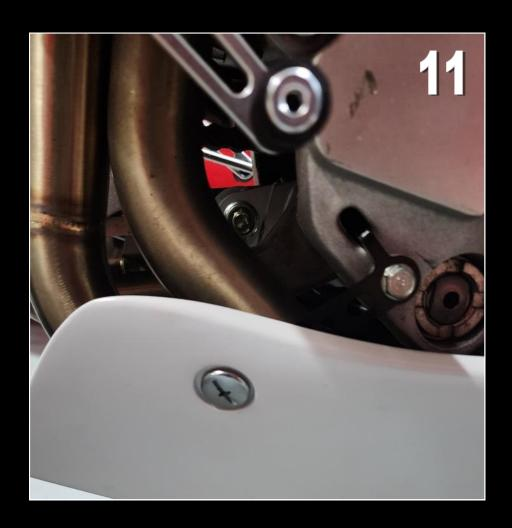
**12)** Fit the bodywork bolt and plastic washer to the lower left stay.
