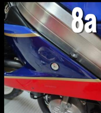
Now to fit the lower cowl. This is quite straight forward but you do need to take care to avoid scratches. I advise to fit the lower from the right hand side of the bike, but first, loosen and move (or remove) the lower left cowl stay, as this can get caught up and possibly scratch the lower if you are not careful and fitting the cowl on your own.
