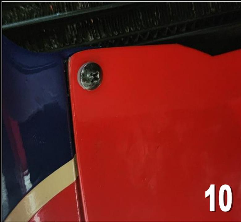
**11)** Fit the bodywork bolt and plastic washer to the lower rear right stay.
