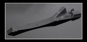
To fit the BPFC/BPCC-7049R In-fill on the VFR750F RC36-2, it is required that the coolant hose that runs from the thermostat housing to the top right spigot on the radiator is shortened by 10~15mm.
