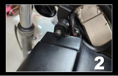
**3)** Fit the M4 bolt and plastic washer to the stay just behind the choke knob.
