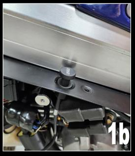
2) Move to the front of the in-fill and secure the in-fill to the radiator stay.
