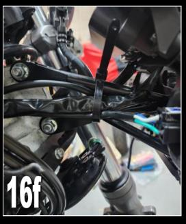
The running light and turn signal wires run over the top of the headlights and down the outer edges. There are hooks on the headlights to retain the wires.
