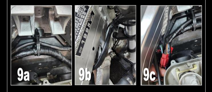
**10)** Now look at the ignition switch wire. For this we need to cut the cable tie that holds the wire to the switch so that we can route it to the left side of the frame and have an adequate length of wire to work with.
