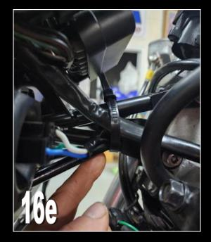
The wires for the running lights and turn signals should route through the meter stay behind the meter, and then split left and right.
