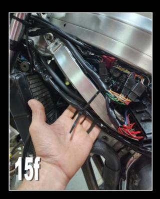
Now run the extension harness on the left side of the meter stay and route it between the meter and the meter stay. Secure to the meter stay with reusable cable tie (provided with meter stay). And finally connect the extension harness and meter stay together and cover up the connectors with the boot.
