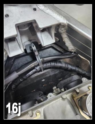
Push the headlight connectors on the extension harness out to the left side of the bike. We do not need to connect up at this stage.
