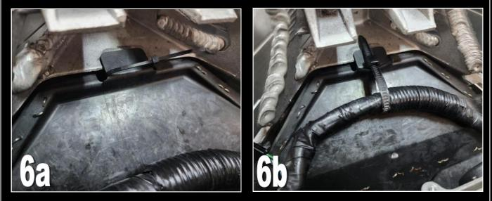
**7)** Now hold the harness as shown, and at an approximate point between the headlight connectors and headlight relay, fold the harness back on itself, and secure the bend with a cable tie.
