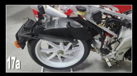
Then you need to lift the front of the undertray up and hook it between the subframe lower left and right spars. The plastic mounts on the undertray are wider than the spars so it takes a bit of a force.
