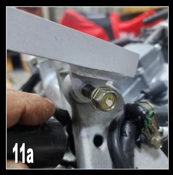
Now is a good time to tighten up a few things. Tighten the upper and lower mounts.
