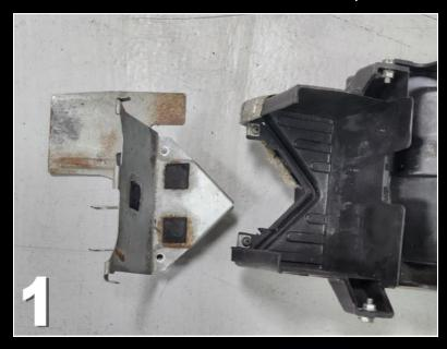
2) Fit the TYLY-0314W Battery Plate. This just drops in and screws on in the same way as the original.
