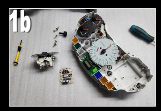
**2)** The electronic module is simply clipped onto the back of the speedo and is removable without tools. There's a couple of little plastic clips, but they can be easy pressed out of the way to remove the module.
