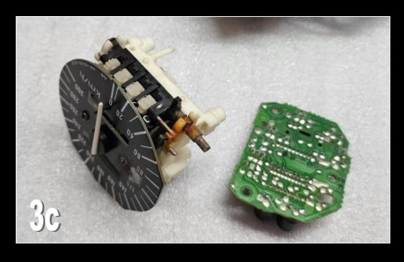
The tachometer is driven by a dual pulse, just like the RC36-2, so no problem there. It is 'almost' plug and play if you are prepared to do a little rewiring.
