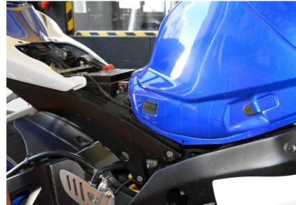
Lift up or remove the fuel tank.
