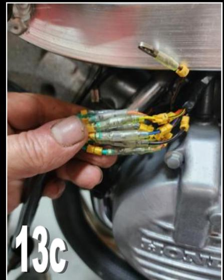
the TYWH-0005 harness does not have the #18 wire for the electronic speedo.
