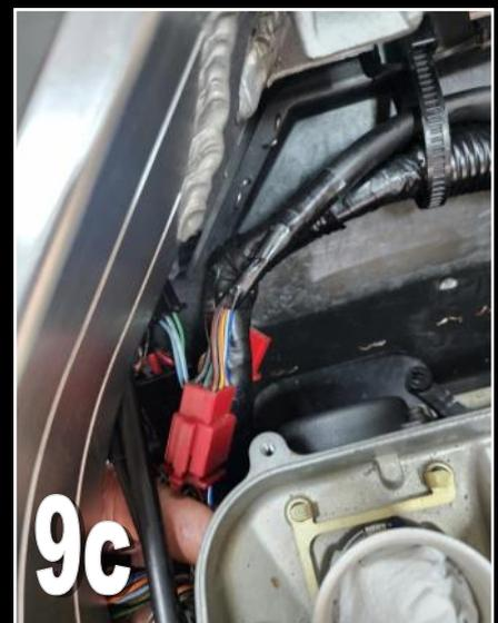
**10)** Now look at the ignition switch wire. For this we need to cut the cable tie that holds the wire to the switch so that we can route it to the left side of the frame and have an adequate length of wire to work with.
