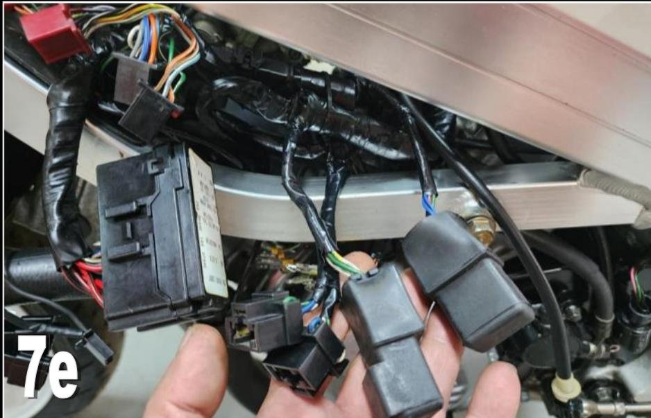
The meter wires and coil wire should be routed from the inside of the lower frame rail and exit on the underside.
