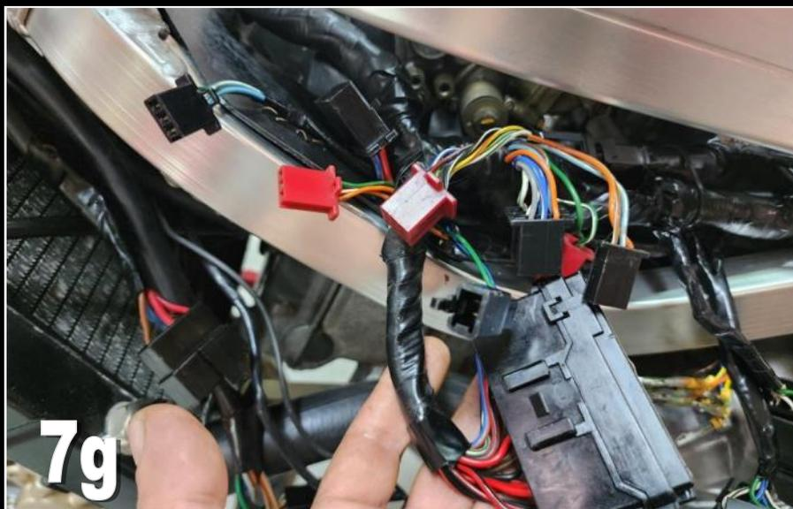
**8)** Locate the 2P fan connector. This needs to run on the inside of the lower frame rail and can be routed under the plastic shield and out to the left of the fame as shown.
