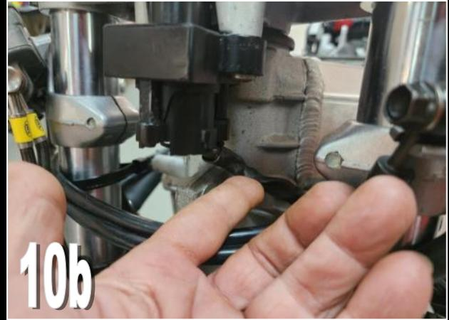
**11)** Route the ignition switch wire on the left side of the fame and connect the plugs as shown
