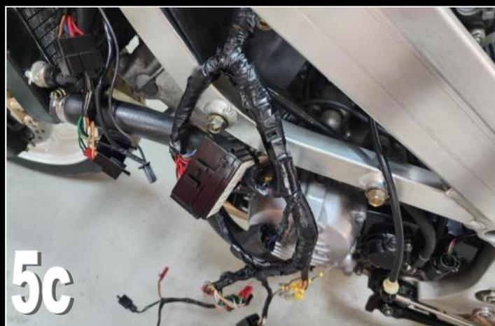
**6)** For wire management, wrap a small cable tie around the front of the plastic shield, and then with a salvaged reusable tie, hold the main harness on position. We will be adding wires here in later steps.
