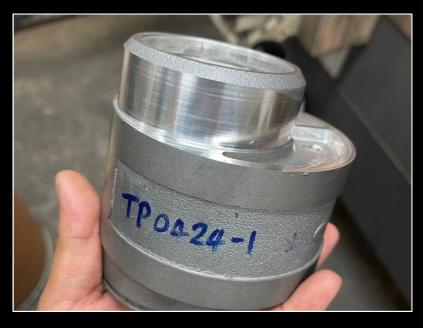
The sprocket carrier nut requires that the 'skirt' is cut off and the nut machined to the same thickness as the RC30 nut. It is then zinc plated to resist corrosion. Note that we do not drill holes in the nut for lockwire, instead we recommend that the nut is fitted using threadlocker to retain it.
