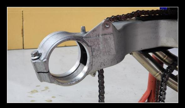
**1)** First job is to fit the stopper TYLY-0326B. This part self locates on the machined step. Secure with the M10x30 bolt. Torque to 35Nm. Insert the split pin through the hole as shown.
