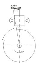
.... i.e. you must enter such an ignition advance value in the "base ignition advance" field which equals to the "base advance" angle (base advance - see the image). The image depicts the top dead centre of the given cylinder. It is recommended to check whether the current advance corresponds with the setting made using the stroboscope lamp.
